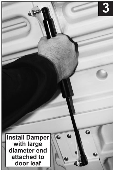
Install Damper with large diameter end attached to door leaf
